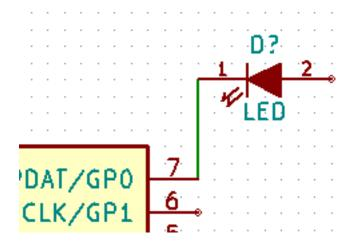
33. Repeat this process and wire up all the other components as shown below. To terminate a wire just double-click. When wiring up the VCC and GND symbols, the wire should touch the bottom of the VCC symbol and the middle top of the GND symbol. See the screenshot below.
